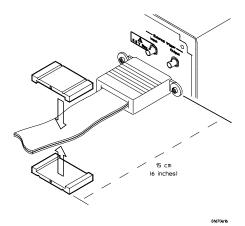
2 Insert the clamps onto the ends of the ferrites. The locking tab should fit cleanly in the ferrite grooves.
