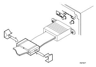
When properly installed, the ferrite should appear on the logic analyzer cable as shown.
